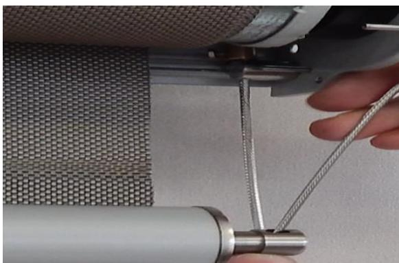
2. Take down the revision lid from the cassette. Then put the cable guide through support in the cassette and bottom bar end cap bolt.
