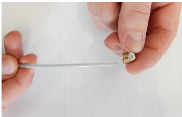
1. Put sleeves on the cable guides . Place a screw in the sleeve, and best with fingers secure it until first resistance, then use flat wrench - and make 2 full turns. Making more turns will damage the screw head.
